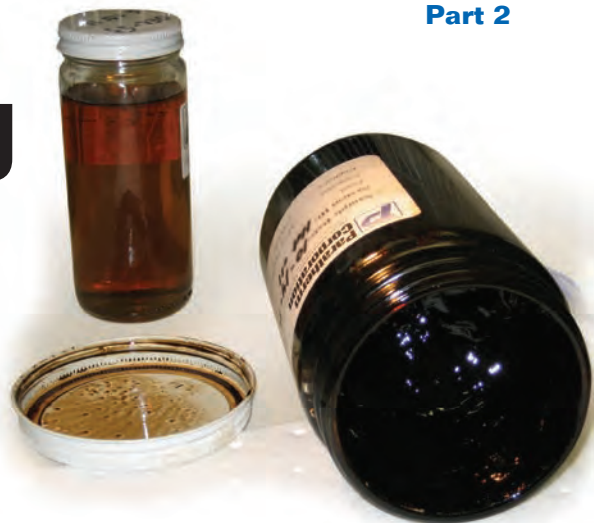
FIGURE 1. A very high viscosity thermal fluid can be a reason for failure of a heat-transfer system
