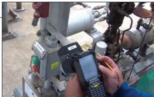
FIGURE 2. The Huntsman wireless mobility application includes mobile handhelds, RFID (radio frequency identification) tags and wireless infrastructure
