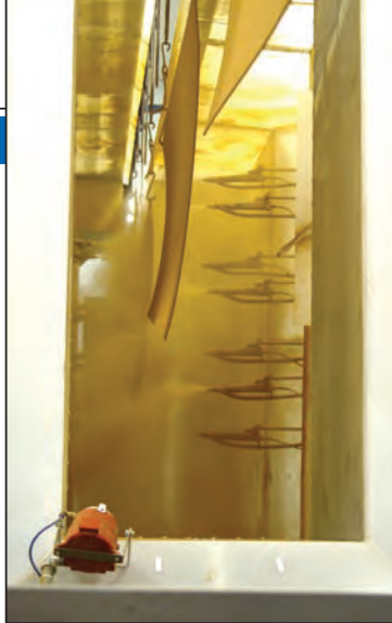
FIGURE 3. Epoxy powder coatings are applied using powder spray guns, which apply a charge to the powder particles when they are atomized. The charge draws particles to the grounded part. The charged particles are preferentially drawn to the thinnest areas and edges, resulting in a uniform coating
