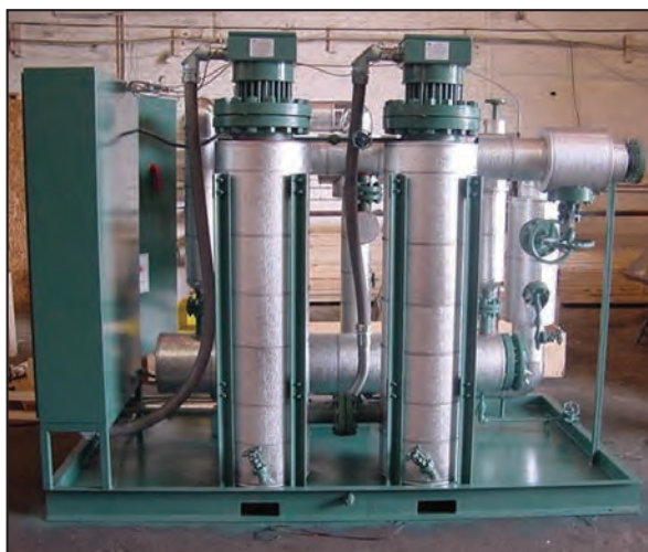
FIGURE 1. This packaged single-fluid system heats fluid directly with the two electrically heated heat exchangers in the foreground. The cooling heat exchanger (horizontally mounted behind the heating units) cools fluid that is diverted through it by a control valve. Fluid is motivated by a pump that is not visible in this image. When installed, this unit will have an expansion tank mounted, either to the unit or nearby
